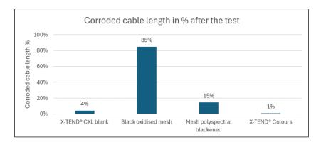
The special polymer coating of X-TEND® Colours forms an additional protective layer that protects the coated material from corrosive animal urine. This increases the service life of the stainless-steel cable mesh, whereas other (mainly chemical) blackening processes impair it.
